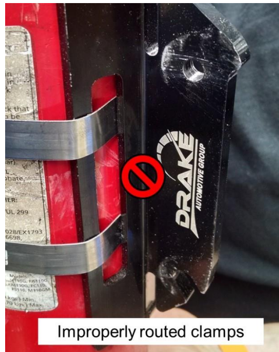
Figure B-48: Incorrect routing of hose clamps.
